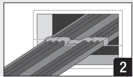
Measure the aperture size and cut the  $3M^{\text{\tiny M}}$  Fire Barrier Composite Sheet CS-195+ to size such that it overlaps past the opening 50mm on each edge. Sheet should be cut to follow the contours of the penetrants as closely as possible.
