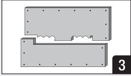
Mark and pre-drill fastener positions in the Composite Sheet, ensuring that each fastener is 25mm from each corner and the maximum spacing between fasteners does not exceed 150mm.
