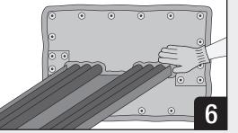
Seal any gaps around penetrants using appropriate 3M<sup>™</sup> Fire Barrier Sealant or 3M<sup>™</sup> Fire Barrier Moldable Putty.
