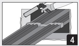
Apply a bead of sealant or putty on the faces of the floor/wall around the opening, 25mm from the edges.
