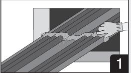
Install appropriate 3M<sup>™</sup> Fire Barrier product to firestop around penetrants as needed per system specs.
